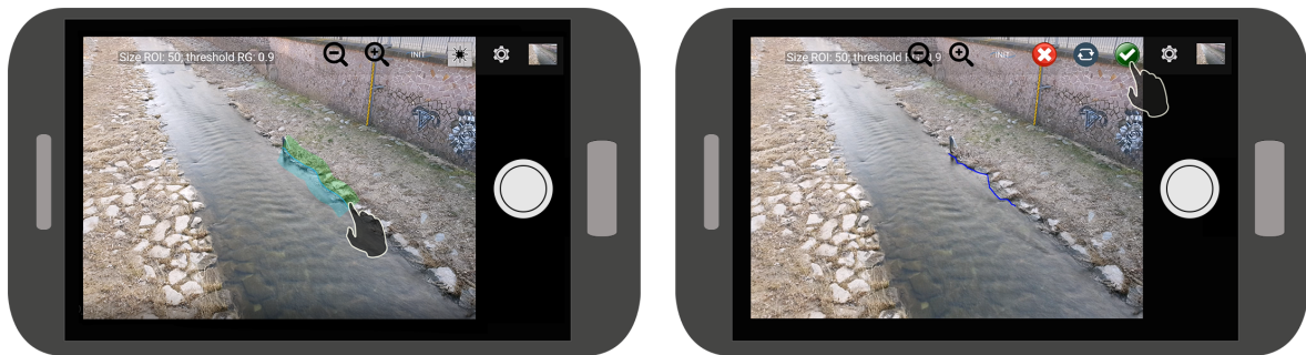
Figure (13.1): Applying OWL for water line detection. Left: ROI definition. Right: Detected water line.
