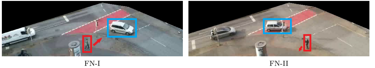
Figure 5.12: Examples of false negative detection on the KoW dataset. The right-turning target vehicles are denoted by the blue bounding boxes and the involved VRUs are denoted by the red bounding boxes.
