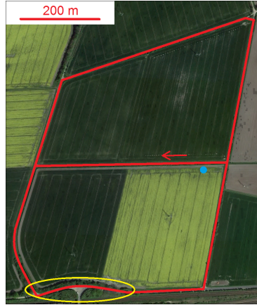
Figure 4.2: Test track of kinematic car experiment: the yellow ellipse depicts a natural alley with signal obstructions, the blue dot indicates the location of the local reference station, the red arrow indicates starting point and driving direction of each eight-shaped test drive (source of map: Google Maps)
