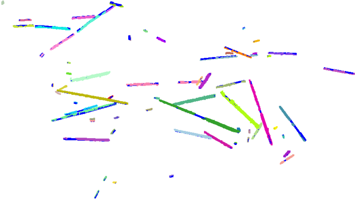
Figure 6.8: All reference tree cylinders derived for Plot A. The dark blue cylinders represent hypotheses from RANSAC, other colors show point clouds of individual trees.
