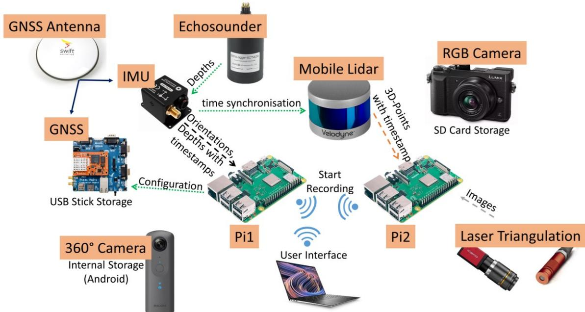
Fig. 2.3: Sensor configuration and system architecture of the multisensory system. The arrow colours indicate different types of connection: dark blue: antenna cable, green: serial port, black: USB, orange: Ethernet, grey: Ethernet (not yet included in the system). The light blue waves indicate a WIFI connection.
