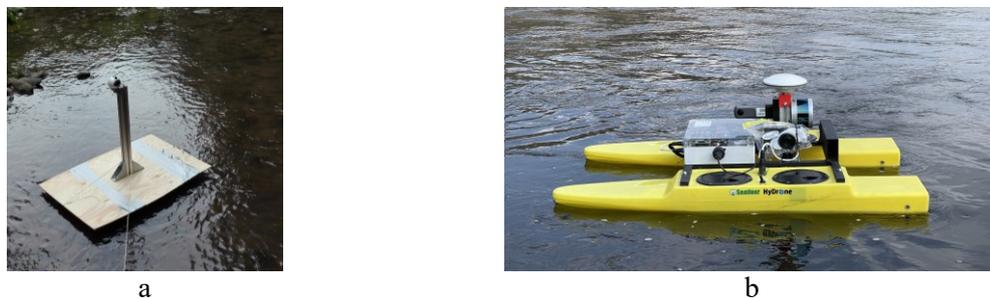
Fig. 2.1: Development stages of the UUV. From a towed wooden board on plastic bottles (a) to a remote controlled multi sensor platform (b).
