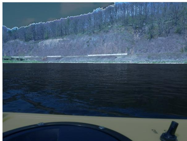
Figure 12: Measurement image used for SfM. Large areas of the image (sky and water) are not suited for matching and therefore masked-out.
