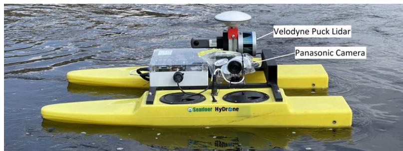
Figure 5: The uncrewed water vehicle used in this study. The Velodyne Puck lidar is attached vertically on the back, while the Panasonic camera is oriented towards the left in the direction of travel, protected with a soft plastic cover.
