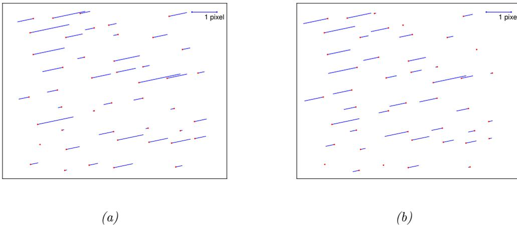
Figure 4.10: Relative pointing error of WorldView-2 data: (a) before RPC refinement (b) after RPC refinement
